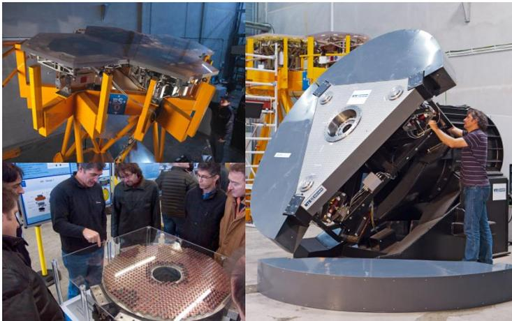
EELT - Prototyping and design of M1 and M5 control systems
