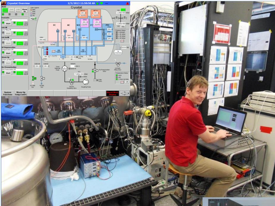
Cryogenic and Vacuum Control System for Scientific Instruments: X-Shooter, Gravity, MUSE, MATISSE
