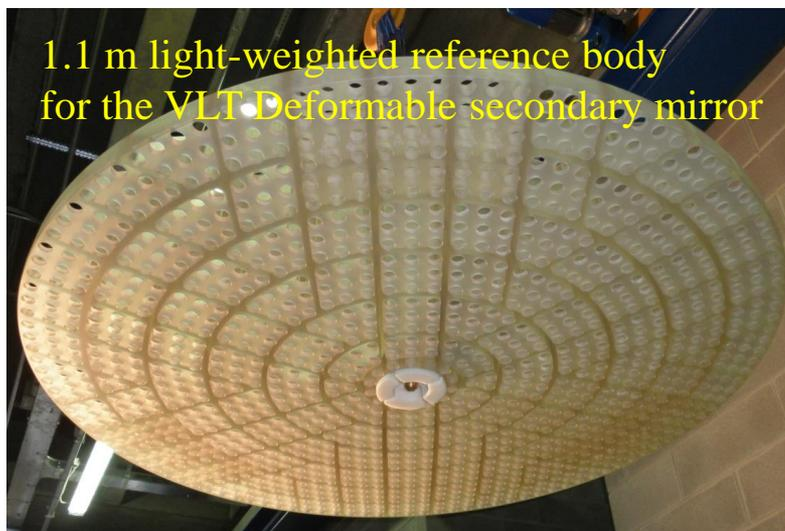
1.1 m light-weighted reference body for the VLT Deformable secondary mirror
