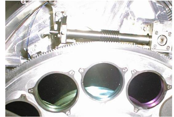
*Custom gears and worm gear system*
