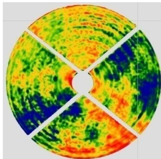
Wave front map for the VLT DMS, best figure: <10 nm RMS
