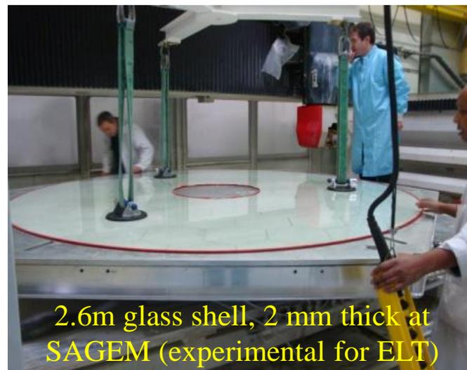
2.6m glass shell, 2 mm thick at SAGEM (experimental for ELT)
